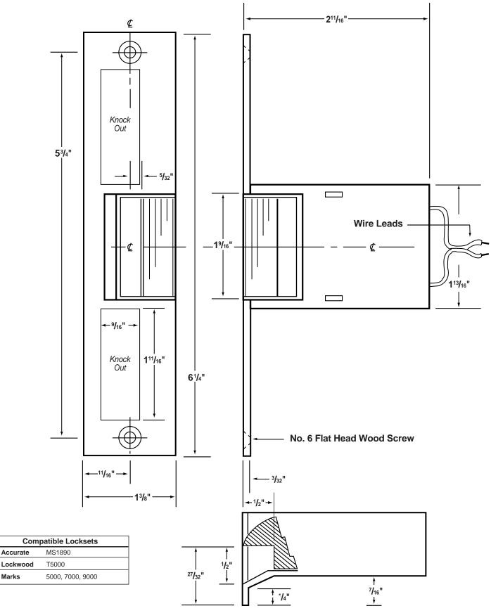
Note: COMPATIBLE LOCKSET designations are offered as a convenience only; reference should be made to manufacturer's catalogs for complete data as to exact equivalents. Caution must be taken in the alignment of locks with latchbolts (only) when used with our electric strike. Lee Electric, Inc. assumes no liability for differences between items compared.
