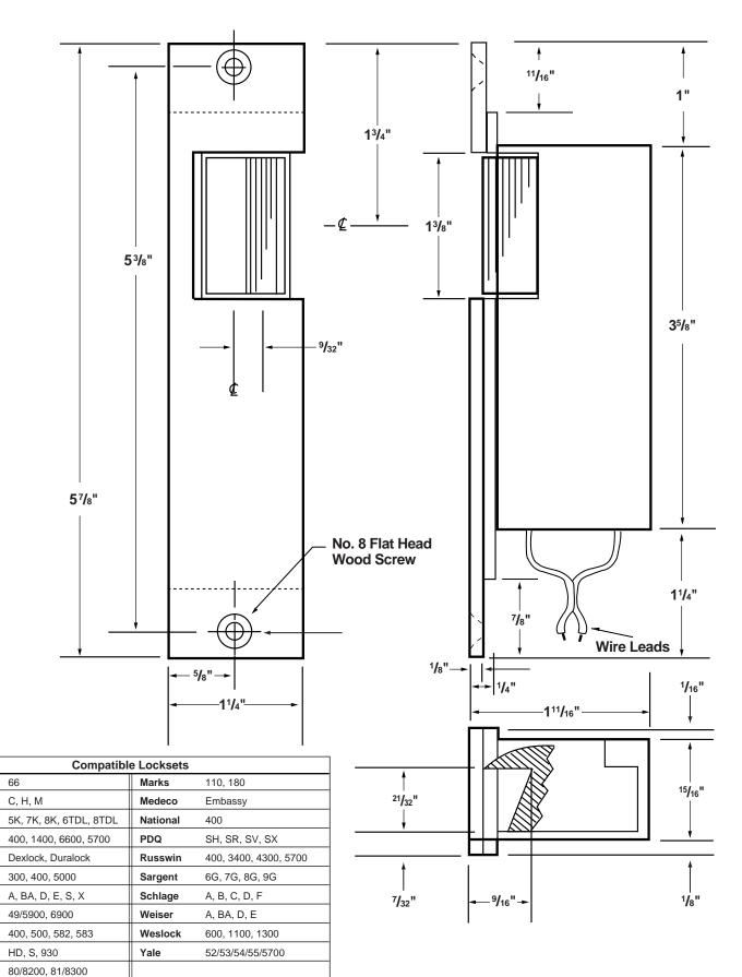
Note: **COMPATIBLE LOCKSET** designations are offered as a convenience only; reference should be made to manufacturer's catalogs for complete data as to exact equivalents. Caution must be taken in the alignment of locks with latchbolts (only) when used with our electric strike. Lee Electric, Inc. assumes no liability for differences between items compared.
